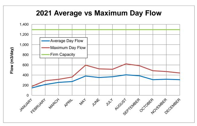
Innerkip Firm Capacity 1,296 m³/day Innerkip Water Supply Capacity 1,296 m³/day
