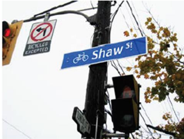
Figure 1 Road Name Plate. Purpose: Identifies the location of a cycling route in a minimalist format to reduce signage clutter.
