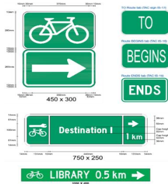
Figure 5 Turn Signs. Purpose: Combined with directional pavement markings to direct cyclists across turns in a bikeway's alignment.
