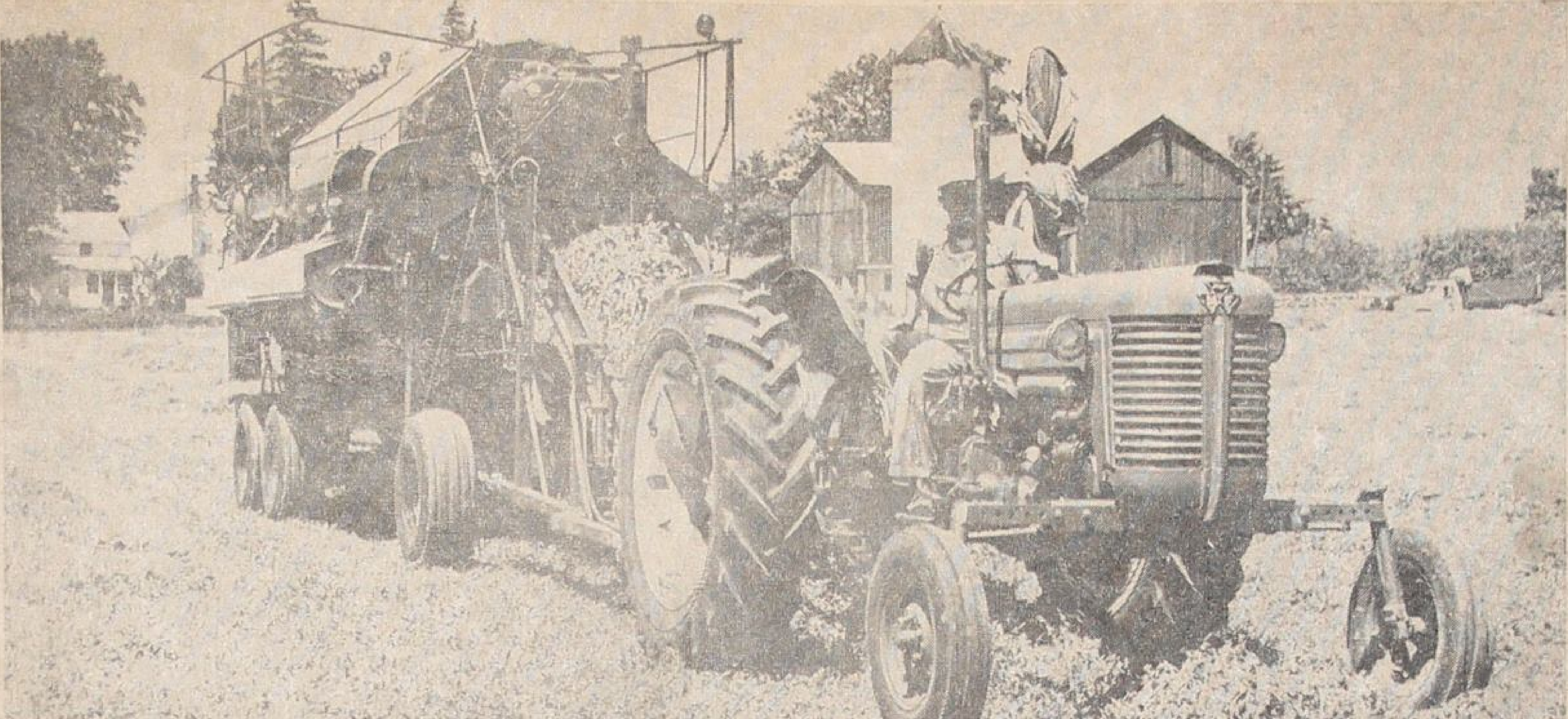
Harvesting peas on the Burgessville farm of Fred B. Griffin, this combine is one of four such machines which will take off the crop for the cannery this summer. The new combines, each worth about $13,000 will be a major change in the traditional method of harvesting the crop. Each unit will harvest and thresh about one-half acre per hour.
