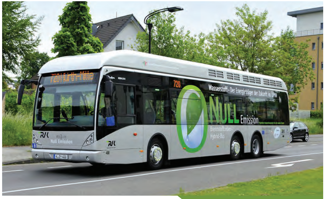
Alternate energy sources, such as hydrogen (above) and high-efficiency battery storage systems, are being developed and tested as possible candidates to replace fossil fuels in intercity bus applications.
