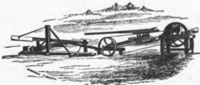
EASTWOOD & CO'S CELEBRATED TWO-HORSE POWER DRAG SAWING MACHINE, WITH STRAW CUTTER ATTACHED.
